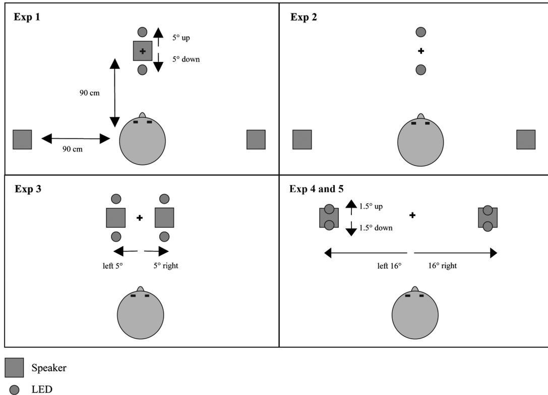
Figure 1. Schematic top view of the setup in Experiments 1–5.
