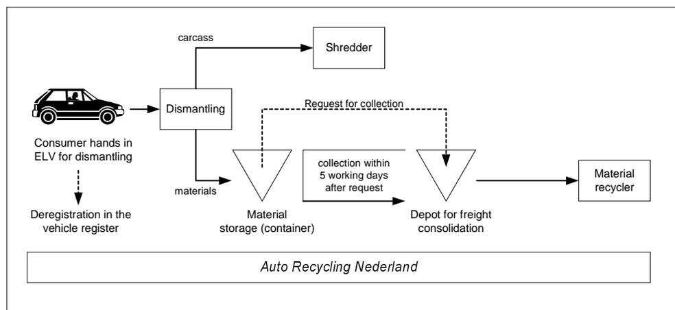
Figure 1. An overview of the processes in the ARN network for the recycling of ELVs
