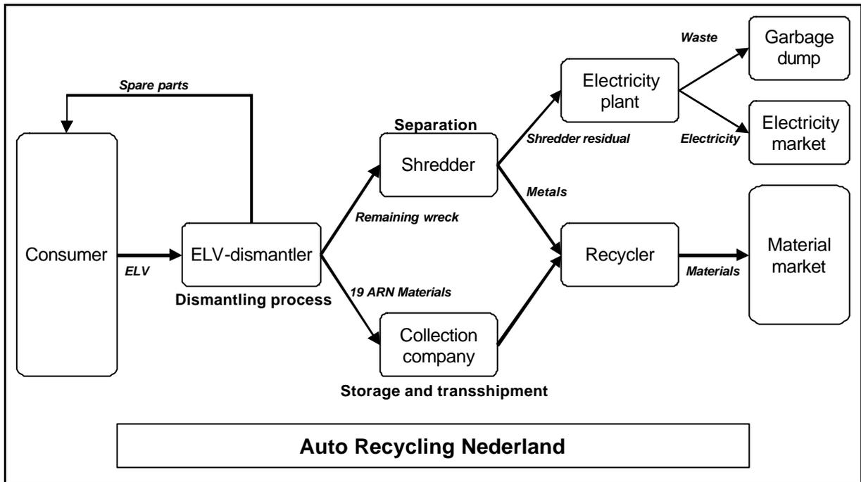
Figure 1. An overview of the ARN chain for the recycling of end-of-life vehicles.
