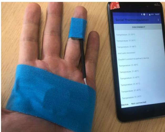
Figure 2. Schematic overview of position of our temperature measurements. Picture of the hand is one of the co-authors and thus posted with consent.
