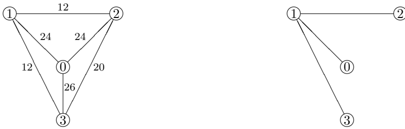
Figure 2.1: An mcst situation \langle \{0, 1, 2, 3\}, w \rangle (left side) and a related mcst (right side).
